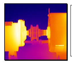
Heat generated from shaft misalignment on the front bearing on the left electrical motor. It is an established fact that a 10°C rise in the normal operating temperature at which the electrical motor functions, the life of the motor is reduced by one half. This damage is irreversible, and can amount to thousands of pounds a year in lost profits.
