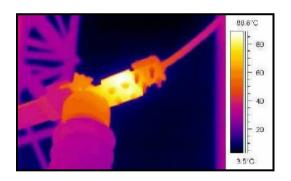
Apart from the costly inefficiency of wasted power, this electrical connection would eventually have resulted in failure once melting point is reached. The cause, a combination of material quality and fixings.
